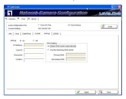
**IP Address**: The IP address obtained at the PPPoE connecting with network.
